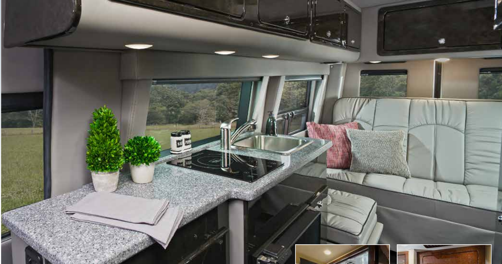
MD4 Lounge with pebble grey solid surface counter top , induction cook top and black burl wood accents.
